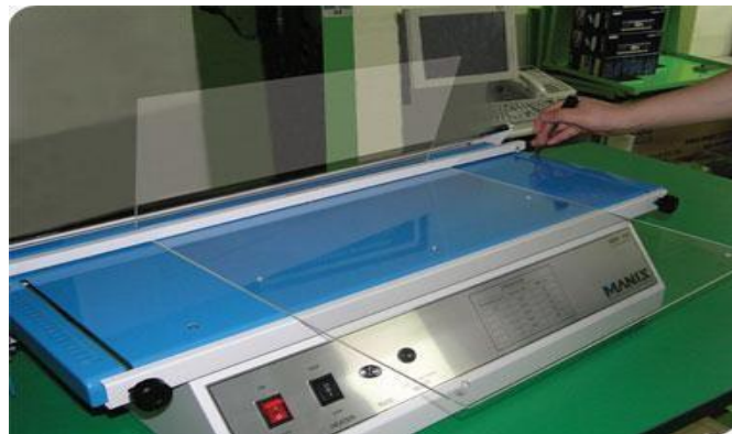
Gambar 2.7 Acrylic bending machine
