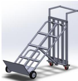
Gambar 2.9 *Hand Truck* Posisi Miring
