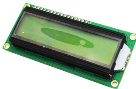
**Gambar 2.4 LCD (*Liquid Crystal Display*)**
