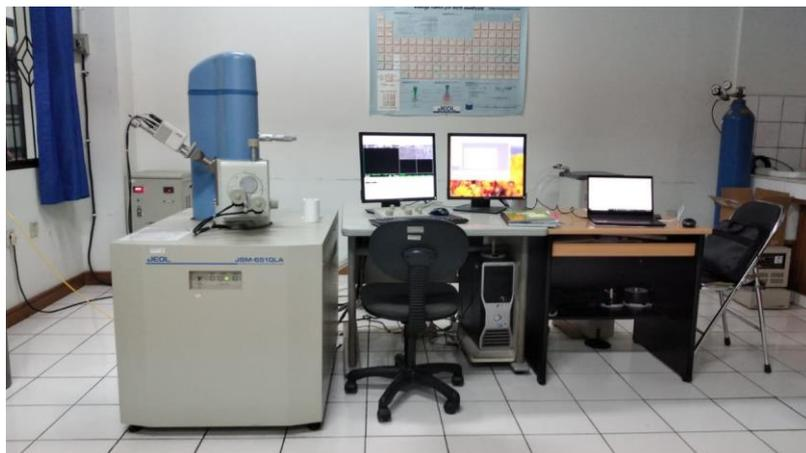
Gambar 3.11 Mesin SEM + EDS JSM 6510 LA
