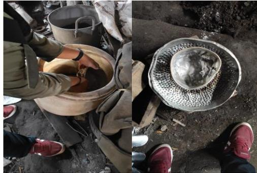
Gambar 3.7 Proses Mencuci Alumunium
