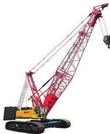
Gambar 2.3 Crawler Crane (Sumber: Lit. 2, 2017)
