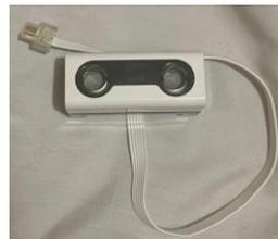
**Gambar 2.15** Sensor Ultrasonik / Sensor Jarak
