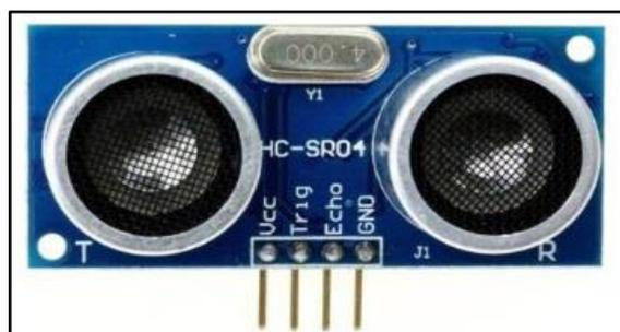
**Gambar 2.14** Sensor Ultrasonik
