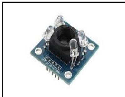
**Gambar 2.14** Sensor Warna TCS3200
