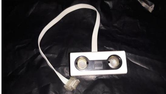
**Gambar 2.5** Sensor Jarak Ultrasonik
