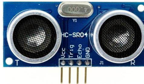
**Gambar 2.8** Sensor Ultrasonik HC-SR04
