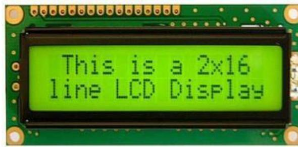
**Gambar 2.13 LCD 16x2**
