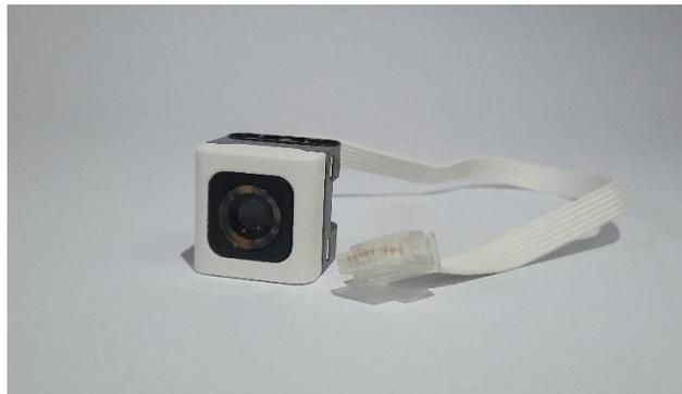
**Gambar 2.4** *Lego Technic Color Sensor*
