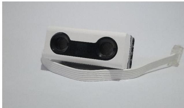
**Gambar 2.6** Lego Technic Distance Sensor
