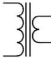
**Gambar 2.13 Skema transformator step-down**
