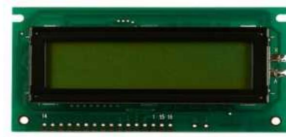
**Gambar 2.3. LCD (*Liquid Crystal Display*)**
