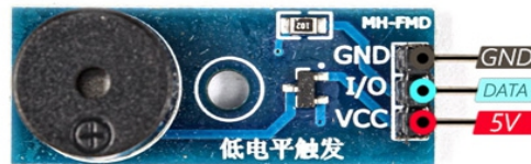
Gambar 3.17 Pinout Buzzer
