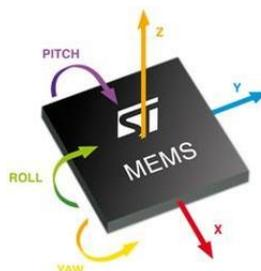
Gambar 2.7 Sensor Accelerometer
