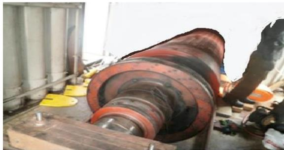
Gambar 2. 27 Rotor Kutub Silinder
