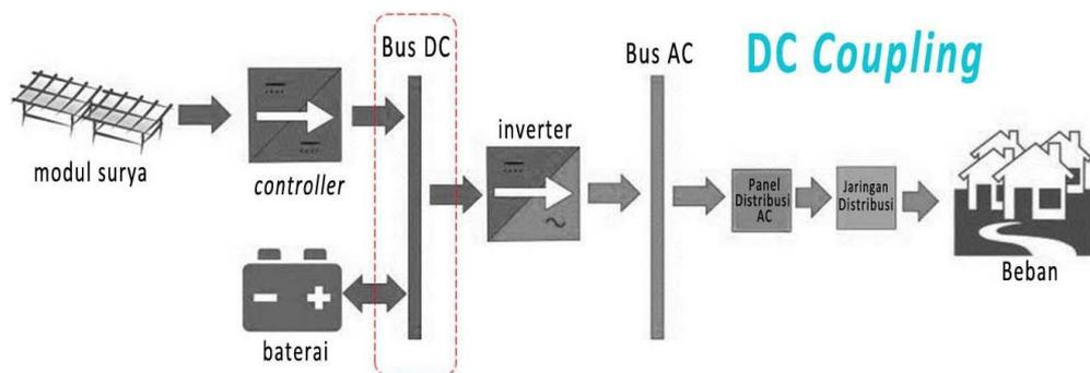
**Gambar 2. 1 Diagram Sistem PLTS *Off-grid* tipe DC Coupling**
