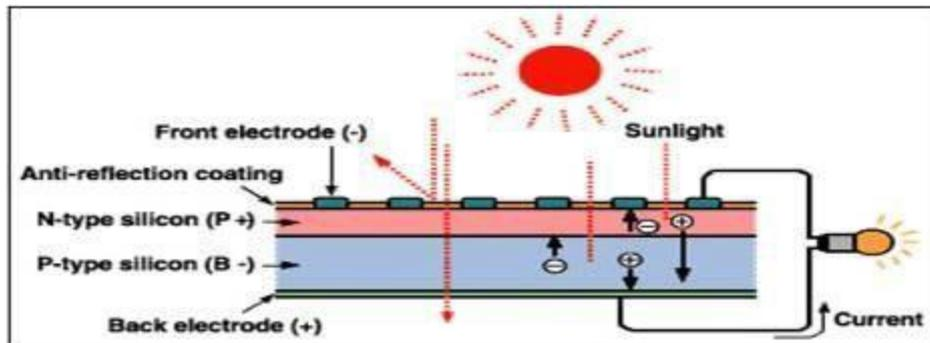
**Gambar 2. 7 Efek Photovoltaic**
