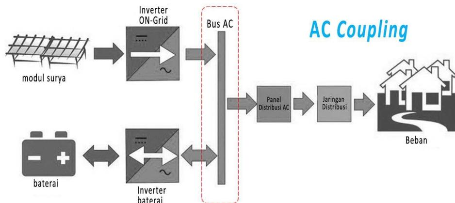
**Gambar 2. 2 Diagram Sistem PLTS off-grid tipe AC Coupling**
