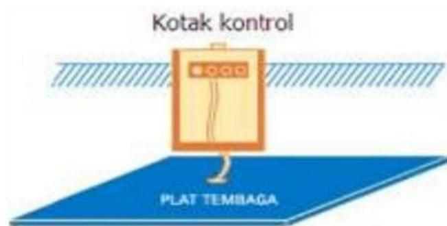
**Gambar 2.5 Elektroda Plat**
