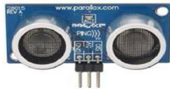
Gambar 2.12 Sensor Jarak Ultrasonik PING
