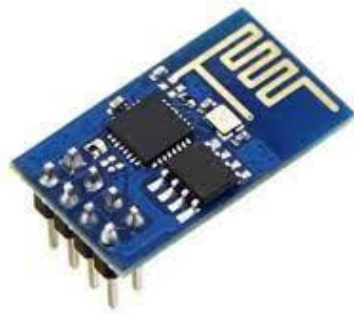
Gambar 2.6 Modul WiFi ESP8266
