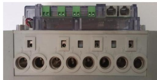
**Gambar 2.3** Kwh Meter Elektronik EDM I type Mk10E
