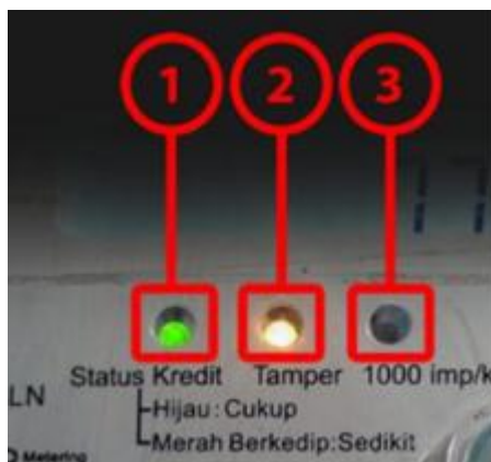
Gambar 2. 6 Indikator Lampu KWh meter prabayar
