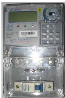
Gambar 2. 10 kWh Meter Merk Melcoinda Type MTS-125 V.1
