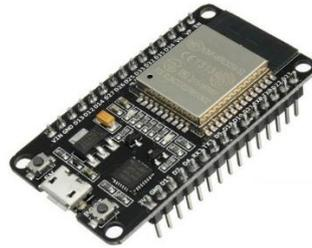
**Gambar 2. 13 NODEMCU ESP32**
