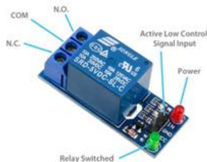
Gambar 2.12 Skema Modul Relay
