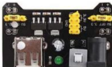
Gambar 2.13 Modul Board Power Supply
