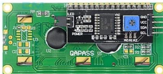
Gambar 2.12 I2C LCD 16 x 2 karakter
