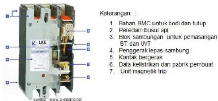
Gambar 2.4 Moulded Case Circuit Breaker (MCCB)
