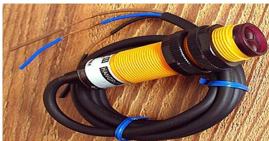
**Gambar 2.22** *Sensor Infrared*
