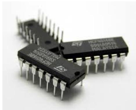
**Gambar 2.12 Integrated Circuit (IC)**
