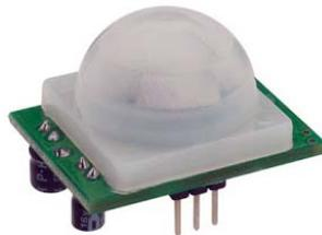
**Gambar 2.18 Sensor Infrared**
