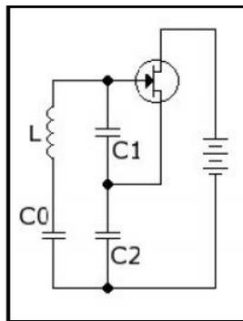
**Gambar 2.5** *Osilator Clapp*
