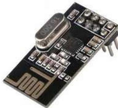
**Gambar 2. 15 Transmitter Receiver Radio**
