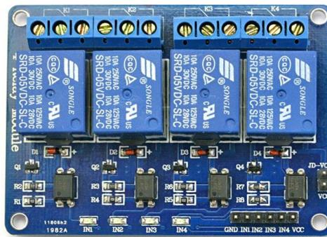
**Gambar 2.10. Modul Relay 4 channel 5 Volt** <sup>[17]</sup>
