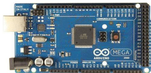
**Gambar 2.6 Arduino Mega2560 [9]**
