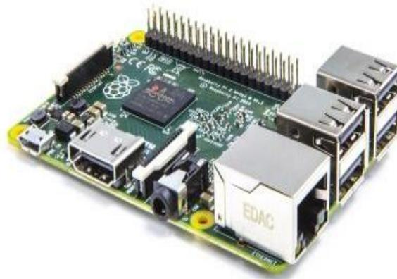
**Gambar 2.7 Raspberry Pi 3 Model B** <sup>[13]</sup>
