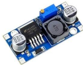
**Gambar 2.5** *Step Down* LM2596 DC to DC
