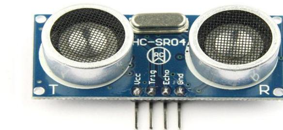
**Gambar 2.9** sensor ultrasonik HC SR04<sup>[12]</sup>
