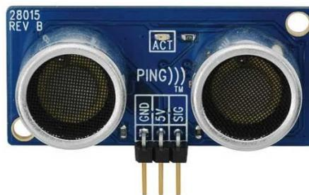
**Gambar 2. 16** Sensor Ultrasonik Ping<sup>17</sup>
