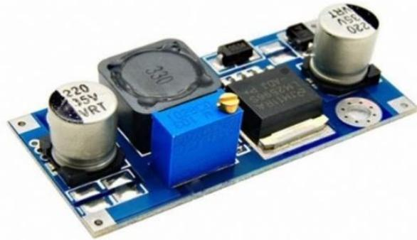
Gambar 2.12 Step Down 5 V 3 A
