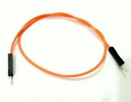
**Gambar 2.18** Kabel jumper *Male to Male*
