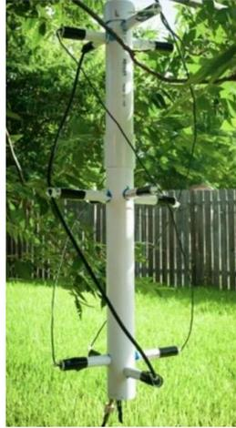
**Gambar 2.7 Antena PVC<sup>[6]</sup>**
