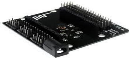
Gambar 2.15 *Shield NodeMCU* (Ahmad Harist, 2016)
