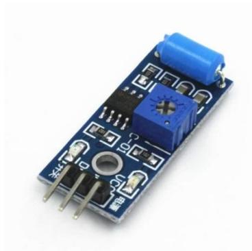
**Gambar 2.10** Modul Sensor Getar SW-420<sup>[16]</sup>
