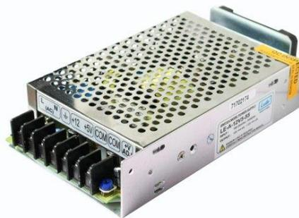
**Gambar 2.10 Switch Mode Power Supply**
