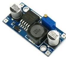
**Gambar 2.11 Modul Step Down Converter LM2596**
