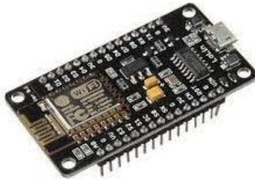
**Gambar 2.2** NodeMCU ESP8266
