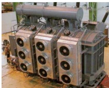
**Gambar 2.19 Pendingin Transformator**
