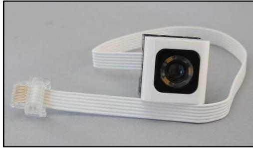
**Gambar 2.16** Sensor Warna Mindstorms 51515
