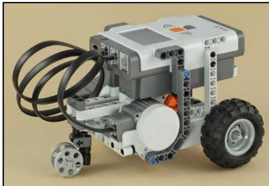
**Gambar 2.2** Robot Beroda (*wheeled car*)
