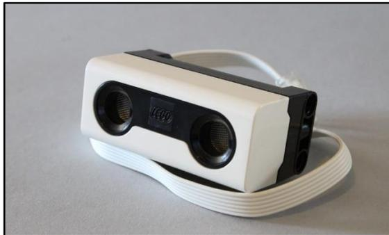
**Gambar 2.17** Sensor *Ultrasonic* Mindstorms 51515
