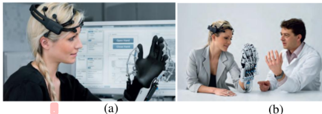
Figure 3. (a) The ExoHand in combination with a brain-computer interface (b) The ExoHand in the rehabilitation of stroke patients
