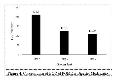
Figure 4 observed that the decrease in BOD content occurring in POME occurs due to the effect of COD decrease. Where the initial BOD content value before getting the processing on the digester of 1.755 mg/liter. The BOD value after processing has decreased to 110.9 mg/liter in tank C as a result of
