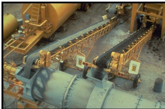
Gambar 2.5 Proses Penambahan *RAP* ke *Drum Plant*
