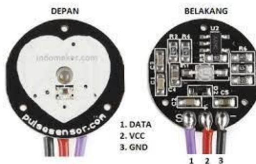
**Gambar 2.1 Sensor Pulse**
