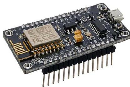
**Gambar 2.5 NodeMCU ESP8266**
