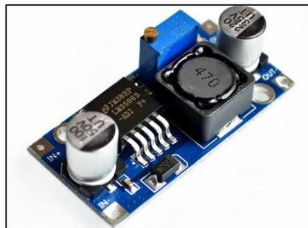
**Gambar 2.8** DC Converter LM2596
