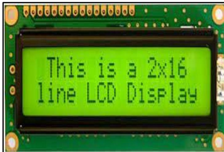
**Gambar 2.14** LCD 16x2
