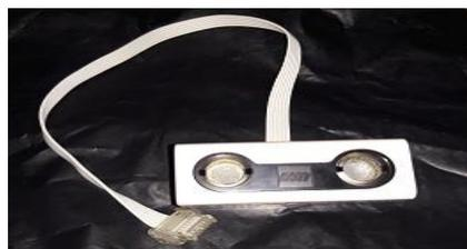
**Gambar 2.20** Sensor Ultrasonik
